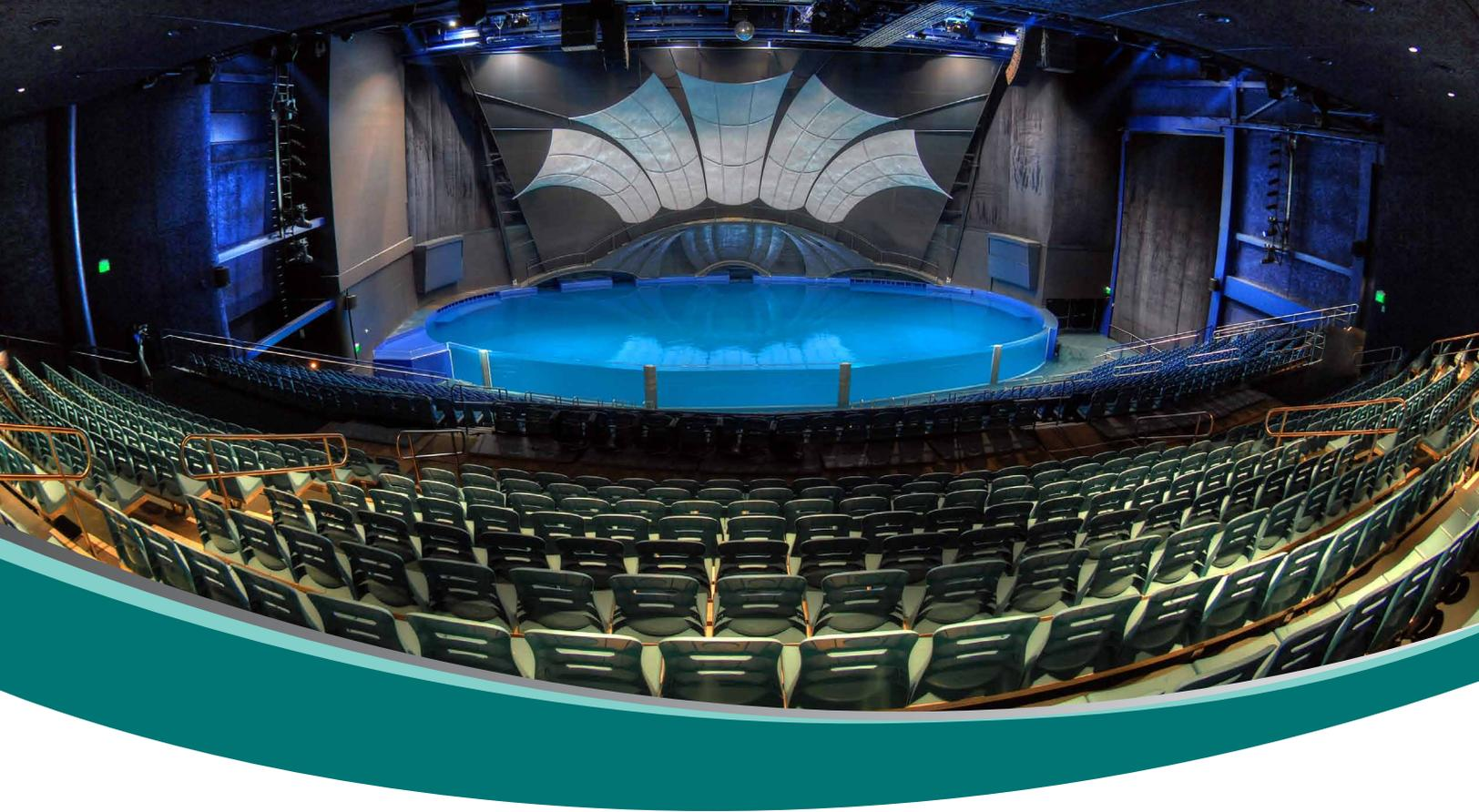
Electrosonic designed a projection system consisting of seven DLP projectors edge-blended in two stacks of three, plus one on center. The center projector forms a flat image on a screen that drops down over the pool in front of the main set. The other screens are the complex curved aluminum structures shaped like dolphin tails. HD media servers handle media playback and content masking on independent video layers, as well as pre-show in-house advertising content and audio playback.
